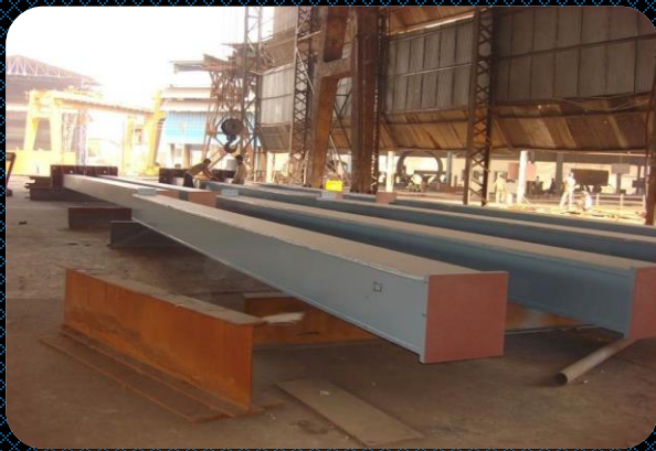
"Box" Columns for Boiler Structures -BHEL
