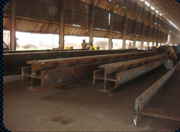
"+" Columns for Boiler Structures -BHEL
