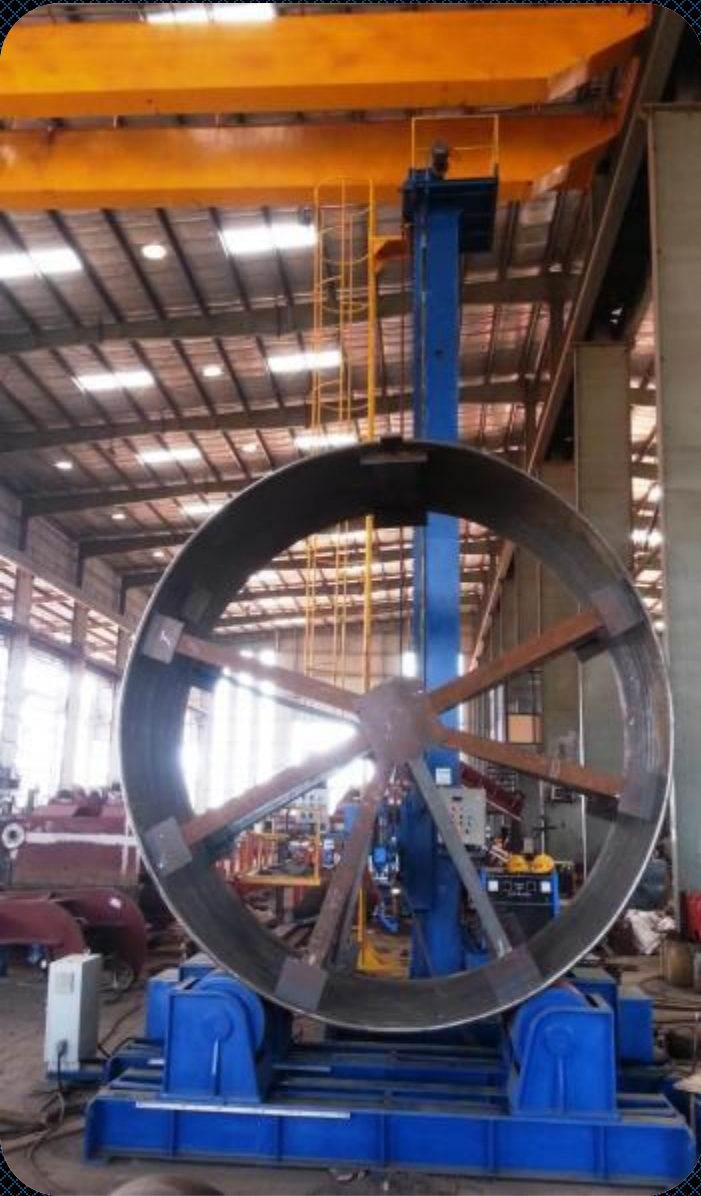
Boom & Colum Welding
